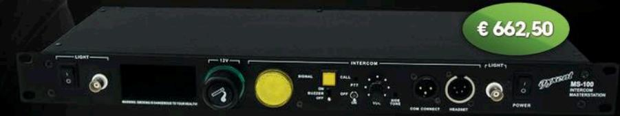
The MS 100 master station provides one intercom channel with high quality audio signal transmission. The power supply of the master station feeds up to 14 belt packs. Sound and light alerts are standard features. All important connectors and controls are located on the front of the unit, such as headset plug, XLR connector for belt packs and XLR line output. All other functions and important data are identical to the two channel unit MS 200 and belt pack BP 100.
